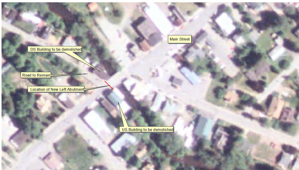
Figure 4.2: Plan View of Proposed Widening of Main Street Bridge
