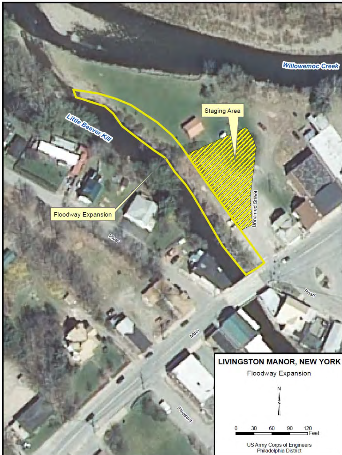
Figure 4.19: Plan H – Widening of the Little Beaver Kill floodplain below the Main Street Bridge.
